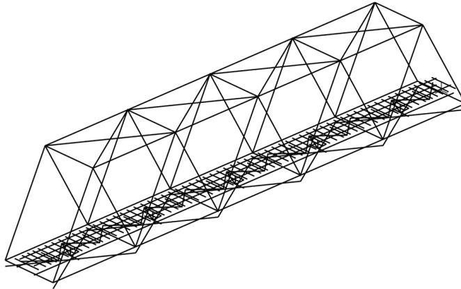
Fig. 10 3D model of the bridge built in ADINA
