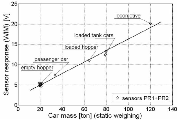
Fig. 7 WIM sensor signals vs. car mass – trend line
