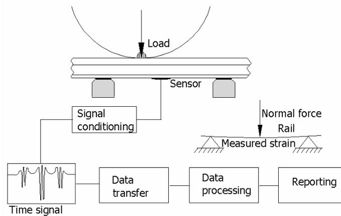
Fig. 5 Data acquisition, transfer and processing in the WIM part of the system
