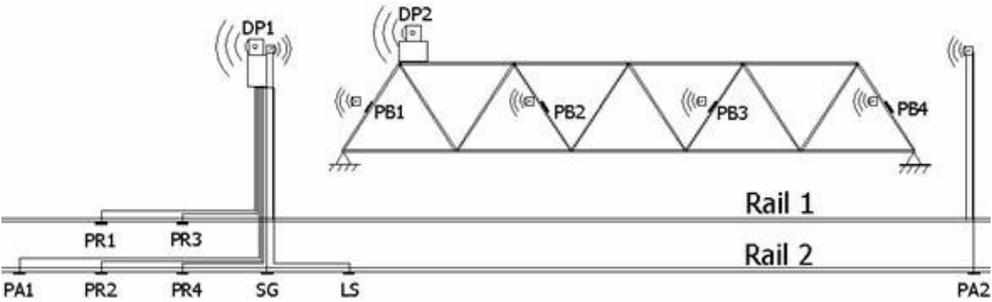
Fig. 3 Layout of sensors mounted for WIM and SHM purposes and scheme of wireless transmission of data:
