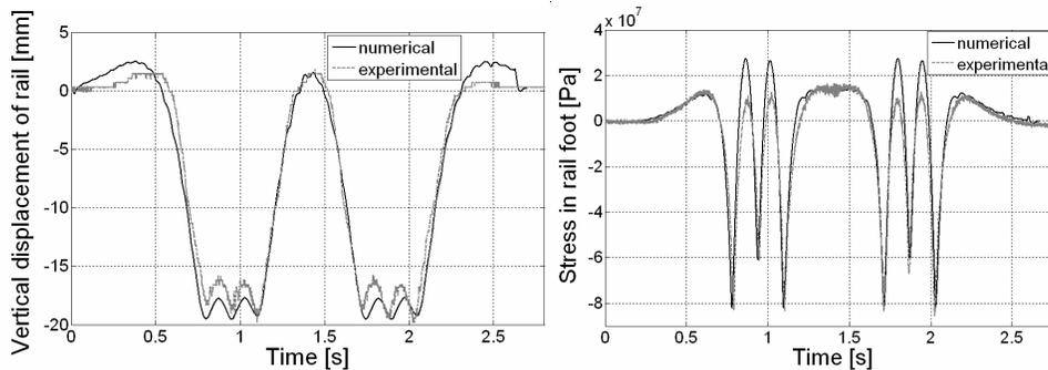
Fig. 9 Numerical vs. experimental results for the WIM part of the system
