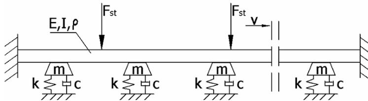
Fig. 8 Model of the rail-sleeper-ground interaction
