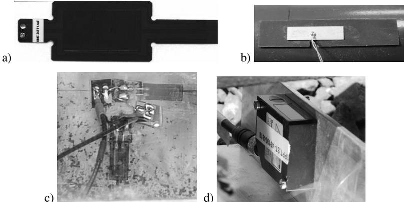
Fig. 4 Types of sensors used: a) PFC, b) PZT, c) strain gauge, d) laser sensor
