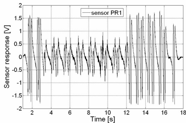
Fig. 6 Time signal collected by a piezosensor during the passage of a freight train
